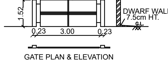
GATE PLAN & ELEVATION
