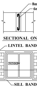
Figure - 3 : Typical Details of Providing Vertical Steel bars in Brick Masonry.
