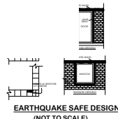
EARTHQUAKE SAFE DESIGN (NOT TO SCALE)
