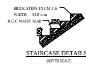
STAIRCASE DETAILS (NOT TO SCALE) TREAD 250 mm RISER 150 mm WIDTH 910 mm
