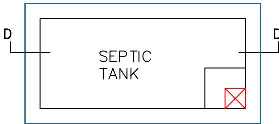
PLAN OF SEPTIC TANK SCALE 1"=2'0"
