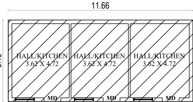
DEMOLISHED GROUND FLOOR MANGALORE TILE ROOF PLAN
