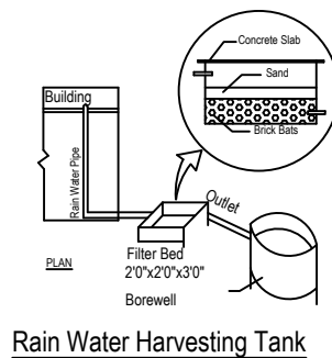
Rain Water Harvesting Tank
