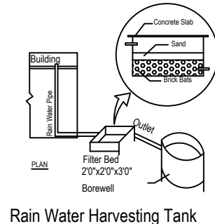
Rain Water Harvesting Tank
