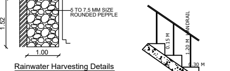
Rainwater Harvesting Details
