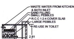
RECYCLING OF WASTE WATER KITCHEN & BATH ROOM
