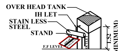
SOLAR WATER HEATING SYSTEM
