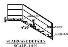
STAIRCASE DETAILS SCALE- 1:100
