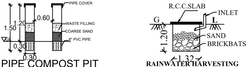
PIPE COMPOST PIT
