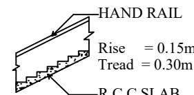
DETAILS OF STAIR CASE
