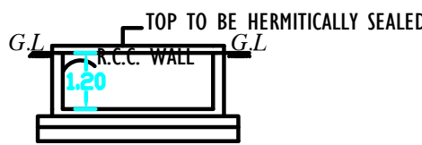
RWH SECTION (SAMPLE)
