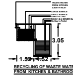
RECYCLING OF WASTE WATER FROM KITCHEN & BATHROOM
