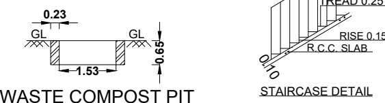
WASTE COMPOST PIT
