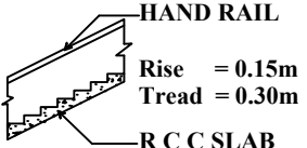
DETAILS OF STAIR CASE
