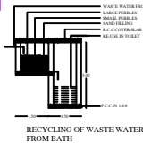
RECYCLING OF WASTE WATER FROM BATH
