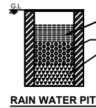
RAIN WATER PIT
