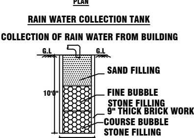
SECTION ON RAIN WATER COLLECTION TANK
