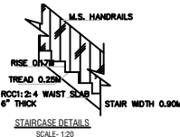
STAIRCASE DETAILS (SCALE: 1/20)
