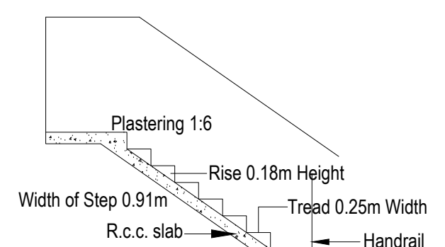
DETAILS OF STAIR CASE
