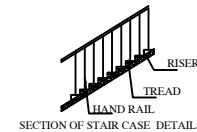
SECTION OF STAIR CASE DETAILS
