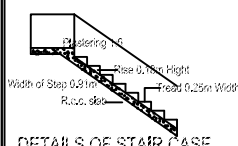
DETAILS OF STAIR CASE
