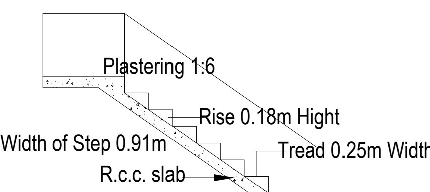
DETAILS OF STAIR CASE
