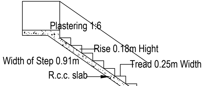
DETAILS OF STAIR CASE
