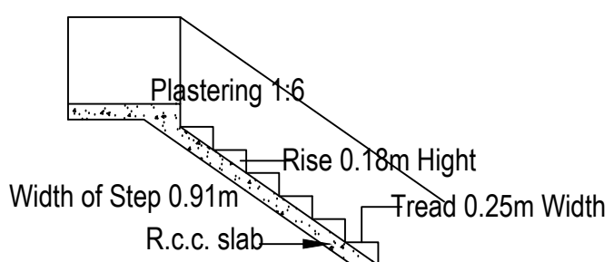
DETAILS OF STAIR CASE
