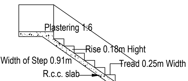
DETAILS OF STAIR CASE
