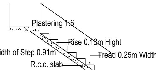
DETAILS OF STAIR CASE
