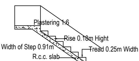
DETAILS OF STAIR CASE
