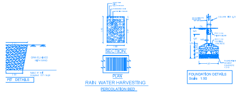
RAIN WATER HARVESTING PERCOLATION BED
