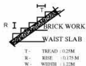
STAIRCASE DETAILS (NOT TO SCALE)
