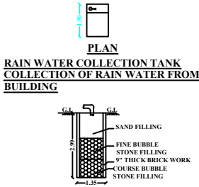
SECTION ON RAIN WATER COLLECTION TANK
