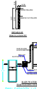
RAIN WATER HARVESTING SYSTEM
