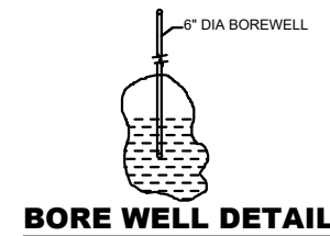
BORE WELL DETAIL
