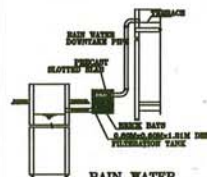
RAIN WATER HARVESTING SYSTEM
