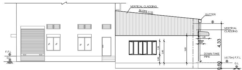
(EXISTING SHOT BLASTING SHED) SPARE COMPONENT PREPARATION SHED
