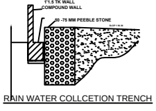
RAIN WATER COLLECTION TRENCH
