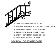
SECTION OF STAIR CASE
