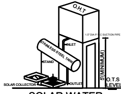
SOLAR WATER HEATING SYSTEM
