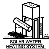
SOLAR WATER HEATING SYSTEM
