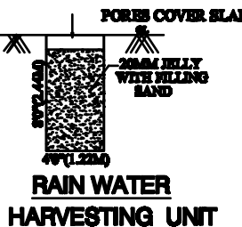
RAIN WATER HARVESTING UNIT
