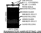
RAIN WATER HARVESTING UNIT
