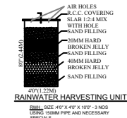
RAINWATER HARVESTING UNIT
