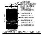
RAINWATER HARVESTING UNIT
