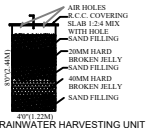
RAINWATER HARVESTING UNIT SIZE: 4'0" X 4'0" X 1'0" - 1'6"
