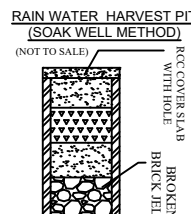
RAIN WATER HARVEST PIT (SOAK WELL METHOD)
