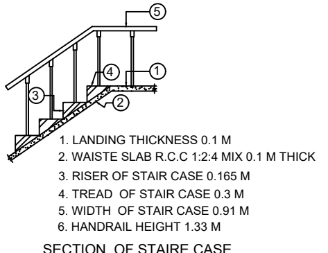
SECTION OF STAIRCASE
