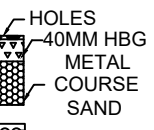
RAIN WATER COLLECTING TANK
